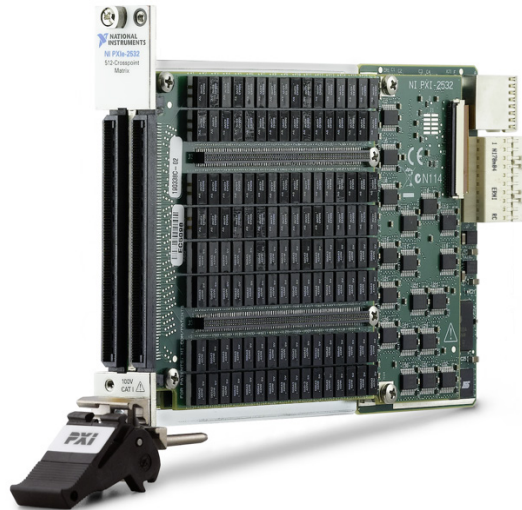
Figure 1. The PXIe-2532B is one example of a PXI Matrix Switch Module that can be reconfigured into various matrix topologies, ranging from a single 4 x 128, 1-wire matrix to a 16-bank 2 x 16, 1-wire matrix.
