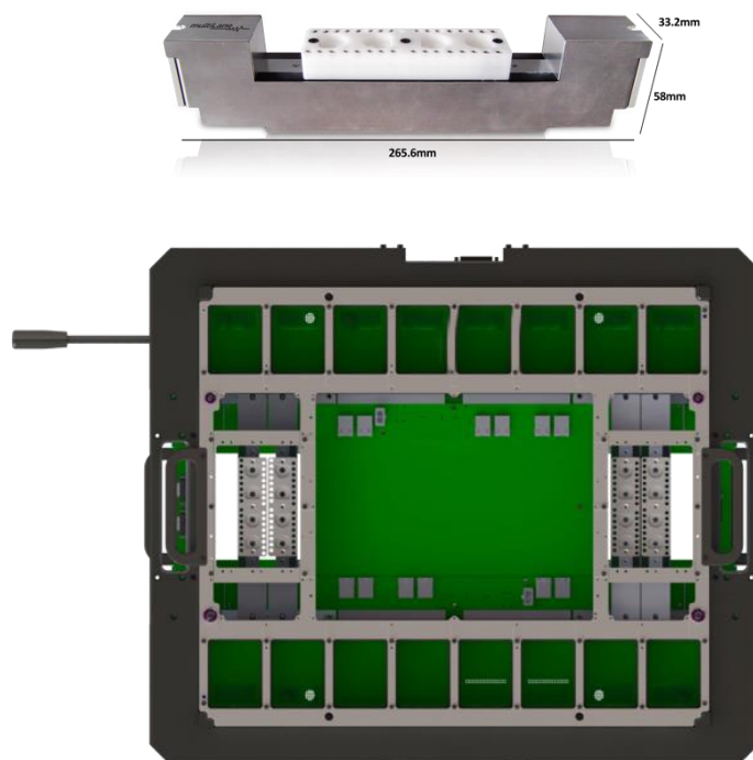
Figure 1: Four ML cassettes mounted in an Advantest V93K HSIO test head extender frame
