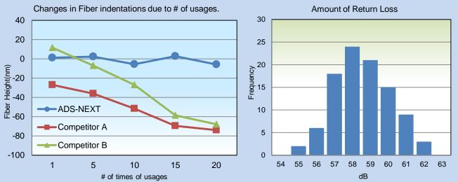
%This data is an example of polishing results. Results are influenced by various factors, such as polishing conditions, the polisher used, and the type of ferrule.
