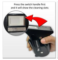
Turn the fiber optic connector end-face to face one of the slot and slowly slide the connector down.
