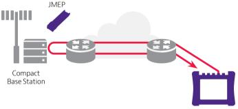
JMEP hot-pluggable transceivers drop in to standards-compliant SFP ports and provide a high-speed serial links at up to 1.25 Gbps signaling rates. They are compatible with the INF-8074i (small form factor pluggable transceiver) standard. An embedded engine performs Ethernet operations, administration, and maintenance (OAM) functions based on industry standards (802.1ag and Y.1731) including test turnup automation, enhanced CPE demarcation, and performance monitoring.
