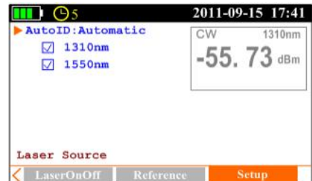
Automatic Wavelength Switch /Identification
