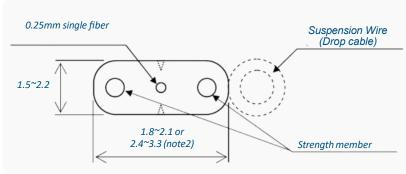
Note 1: Bend insensitive SM fiber must complywith ITU-T.G.652B, G652D and G652A. Allowable fiber diameter is 0.25+/-0.015mm.
